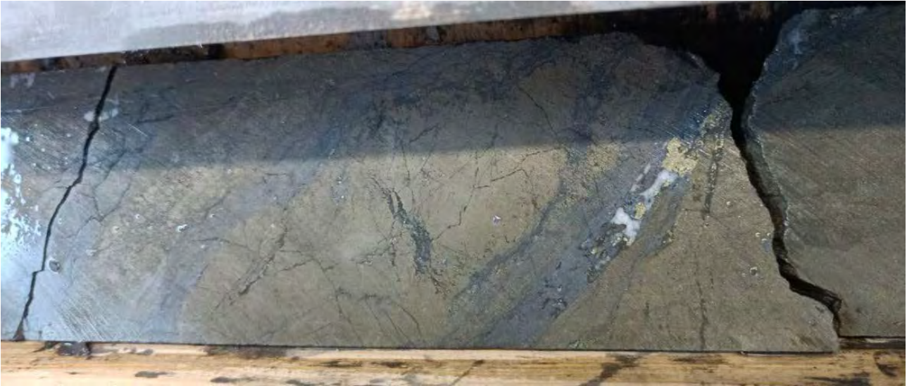
Figure 6. Core photo of EC015 zinc-lead-dominant massive sulfide with cross-cutting high-grade chalcopyrite-quartz veins.
