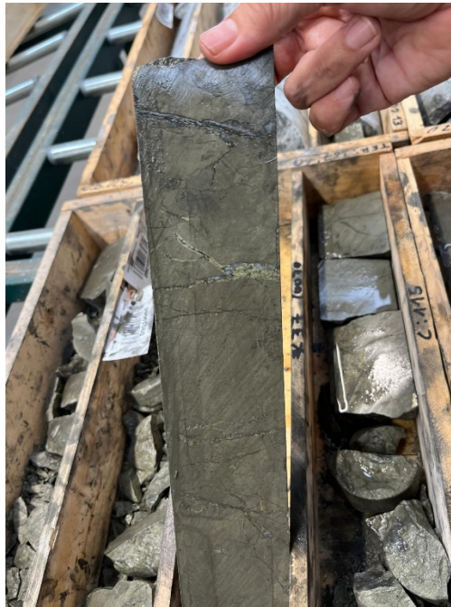
Figure 5: core photo of drillhole EC014 disseminated sphalerite, galena and chalcopyrite in a pyritic mass crosscut by chalcopyrite veinlets.
