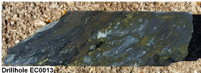
Figure 5: Core photos of drillholes EC012 and EC013 with abundant presence of Chalcopyrite, Sphalerite and Galena.
