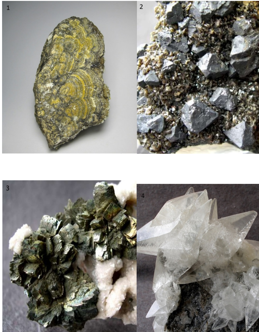
Figure 26: Reocin Samples: (1) Sphalerite, (2) Galena, (3) Marcasite, (4) Calcite .(mindat.org)
